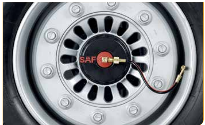
Permanent monitoring of the tyre pressure
